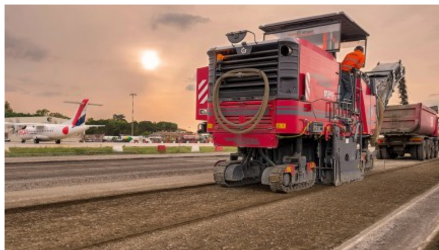
One of the invaluable features of the Wirtgen W 200 is Wirtgen's proprietary PTS ("Parallel To Surface") system, which automatically aligns the machine parallel to the road surface in a dynamic process: The front and rear crawler units are lowered evenly and parallel to one another. In addition, the 4-fold full-floating axle, which forms part of the PTS system, quickly balances out any unevenness on the left or right side.
