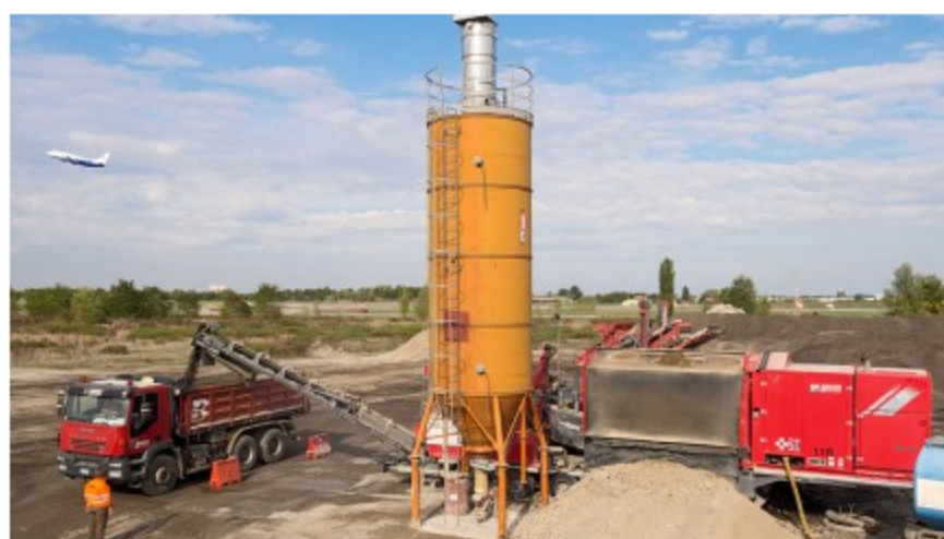
The Wirtgen mobile cold recycling mixing plant KMA 220 is easy to transport and can be quickly set up in the direct vicinity of the job site. That saves time and truck capacity, as well as being very environmentally friendly. It has its own diesel engine to guarantee independence of the public grid.
